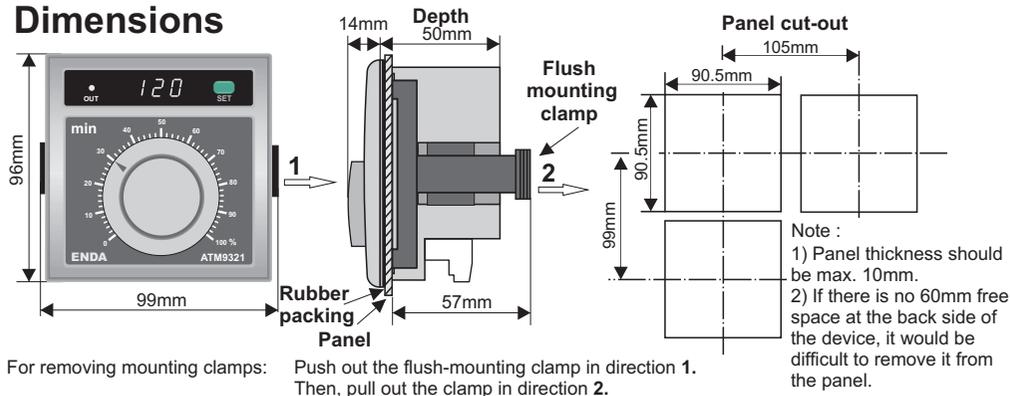
For removing mounting clamps: Push out the flush-mounting clamp in direction 1. Then, pull out the clamp in direction 2.
