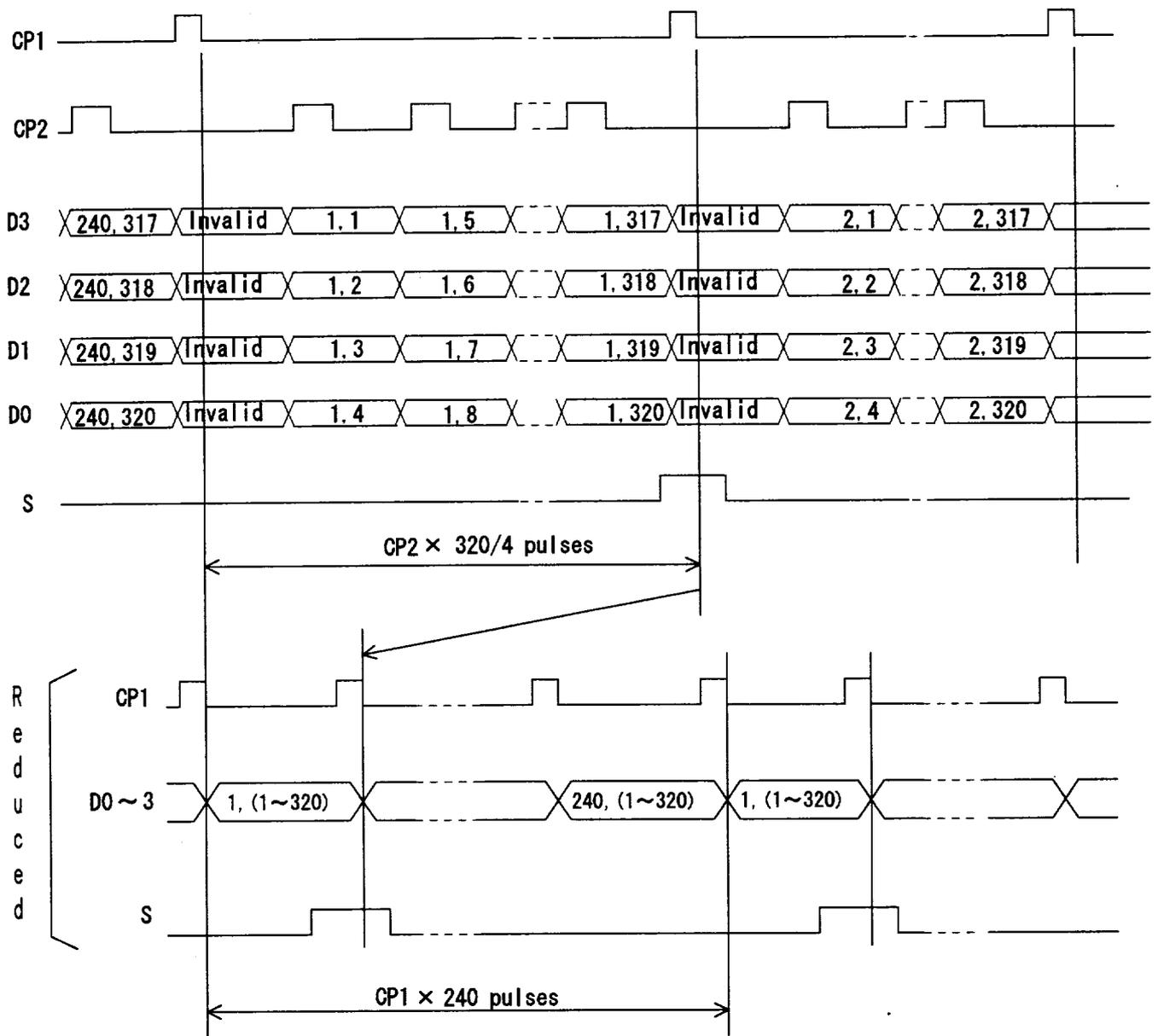
Fig. 2 Data input timing chart
